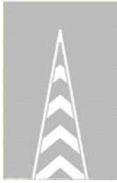
Motorway Slip road markings
